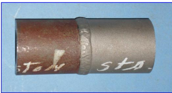
Figure 1. Metallurgical tube sample section representing dissimilar metal weld joint of stainless steel material to lower-alloy steel material. As can be seen above, it is at this type of weld location that any failures occur as a result of the temperature induced stress, carbon diffusion and oxidation resistance.]
