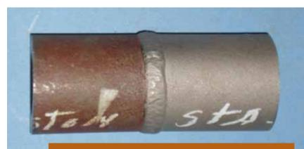
A metallurgical tube sample section representing dissimilar metal weld joint of stainless steel material to lower-alloy steel material. It is at this type of weld location that many failures occur as a result of the temperature induced stress, carbon diffusion and oxidation resistance. Photo courtesy of Thielsch Engineering
